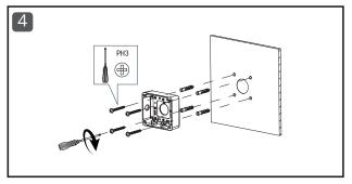
Pull each wire through the cable opening and connect. Next, resecure the mounting plate. See optional procedures A and B to create a more secure attachment for these components.
