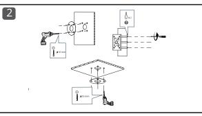
Remove the mounting plate's protective film. Secure the mounting plate onto the camera.
