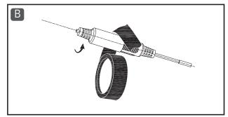
Position and secure the camera at the desired angle. The camera can be moved up and down and rotated. Use the T15 screws to set the camera at an angle or use the S5 screws to set the camera straight vertically or horizontally.
