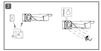
Install the mounting plate and camera (camera not pictured in diagram) onto the desired location.
